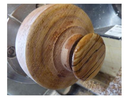
Thin parting tool used to separate pendant – also allows greater access to back for sanding and finishing
